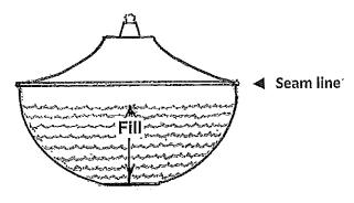
2. Fill Lamp with oil below seam on lamp to insure no leaking. Insert Wick.
